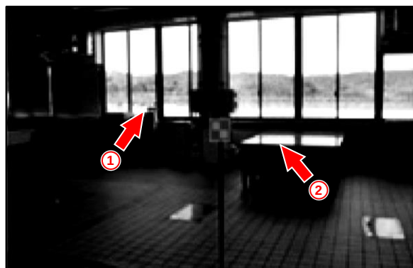
Figure 12. In the Image Processed by the Camera, the Difference in Contrast Between the Target and Objects in the Background is High
